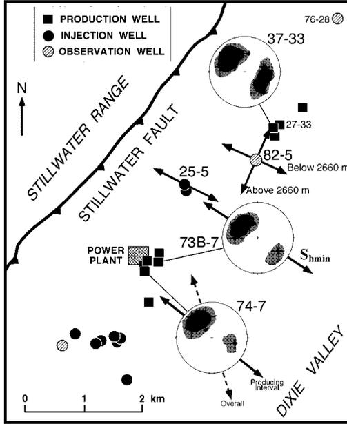
Figure 5. Map of the Dixie Valley Geothermal Field, showing the orientation of  $S_{hmin}$  as outward-directed arrows. Also shown are lower hemisphere stereographic projections of poles to permeable fractures in selected production wells, contoured using the Kamb method (see Figure 8), demonstrating that these fractures and the overall Stillwater fault zone are well oriented for normal faulting in the current stress field (see Barton et al., 1998; Hickman et al., 1998).
