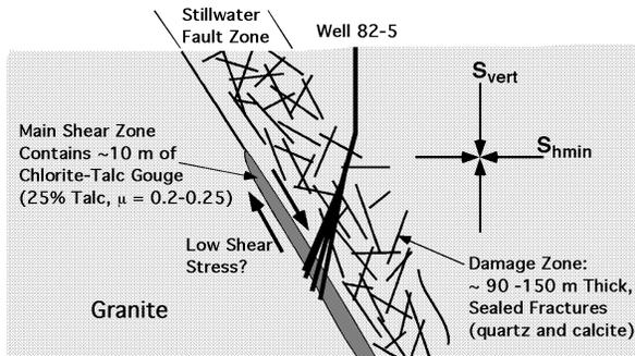
Figure 9. Illustration of the stress shadow model, in which a chlorite-talc gouge with a low coefficient of friction ( $\mu$ ) confined to the main shear zone of the Stillwater fault might lead to anomalously low shear stress on fractures within the adjacent damage zone.
