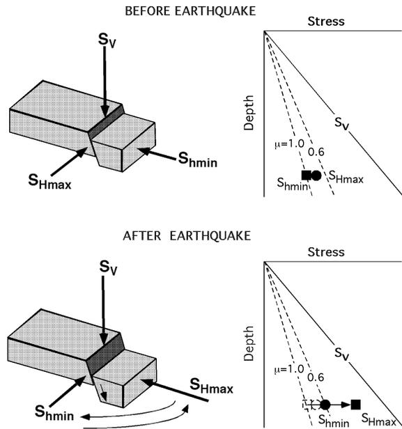
Figure 7. Illustration of the manner in which a normal-faulting earthquake accompanied by a large decrease in shear stress (stress drop) on the causative fault could lead to a 90° flip in the orientation of the two horizontal principal stresses.
