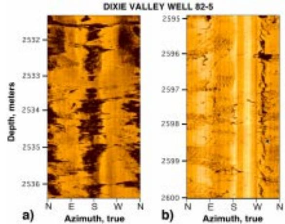
Figure 3. Borehole televiewer log from well 82-5 showing: (a) borehole breakouts (irregular dark patches) and (b) drilling-induced tensile cracks (undulating vertical features) on diametrically opposed sides of the borehole. Several natural fractures can also be seen in (a) as sinusoidal dark lines (e.g., 2531.5 m).
