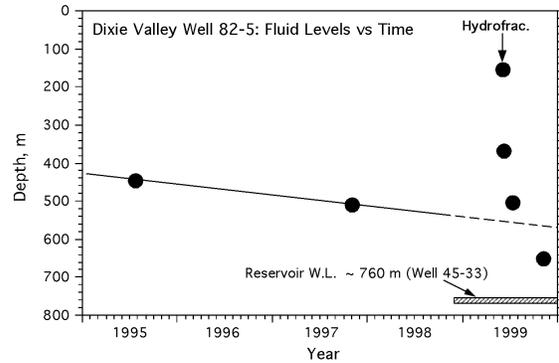
Figure 10. Water level in well 82-5 before and after the hydraulic fracturing test, compared to the static reservoir level in nearby production well 45-33.
